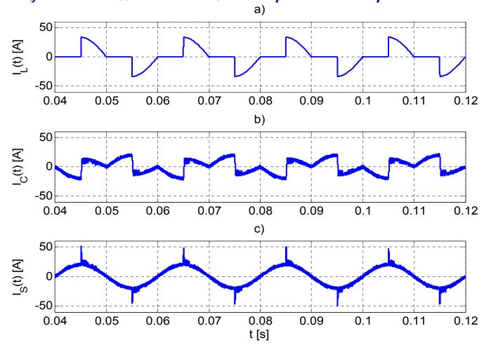
$L_{Cf}$  =0,2mH,  $L_{Cs}$  =1,5mH,  $U_{DC}$  390V,  $f_{p2}$  =51200 Hz,  $f_{p1}$  =25600 Hz
