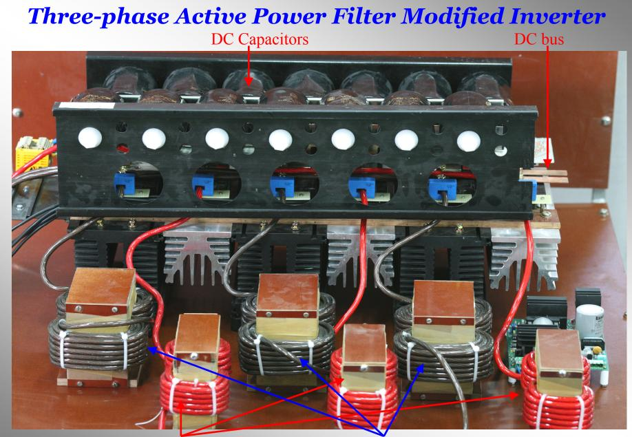
Inductors for high frequency switches
